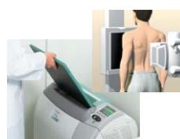
Image data stored on an Imaging Plate (IP) are read by a reader unit. An IP can be used repeatedly since the image data can be erased.
